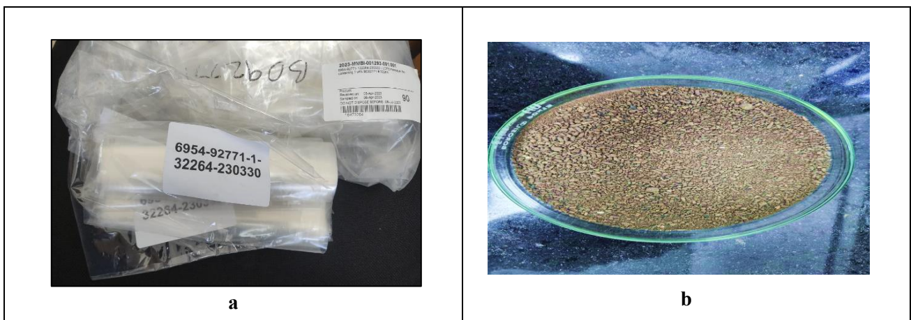
Figure 1: a. Original sample – Polyethylene films containing 1wt% Reverte BD 92771 b. Resulting Biomass after testing for ASTM D6954-24
